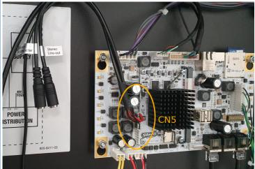
The following machines equipped with a SPIKE2 system have only 6 pins on their CN5 connector:
